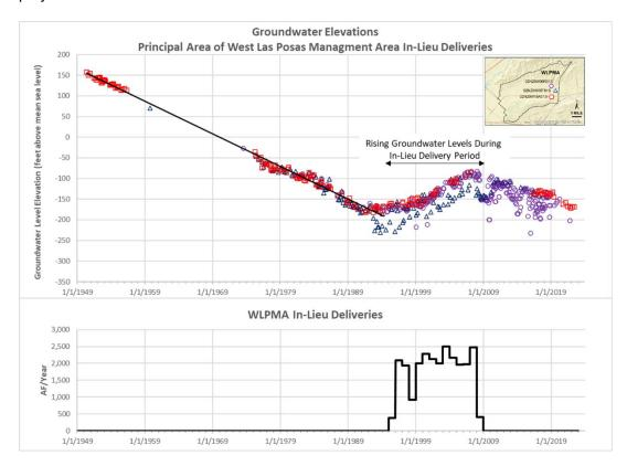
Historical data demonstrates that a similar magnitude of in-lieu deliveries to WLMPA between 1996 and 2008 resulted in groundwater elevation increases of approximately 90 feet, as shown in the charts above.
